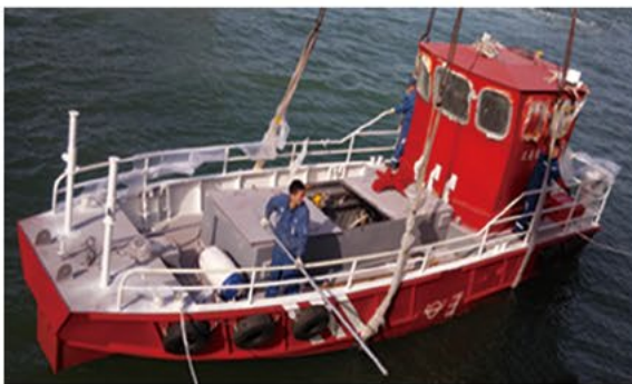
电磁流体海面浮油回收分离技术装置 Electromagnetic Fluid Seawater Floating Oil Separation And Recover Equipment
