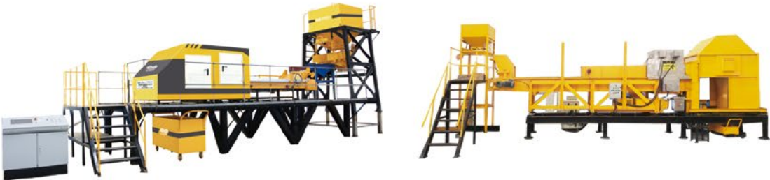
X射线智能传感分选机 HRS- X-ray sensor based intelligent sorting system
